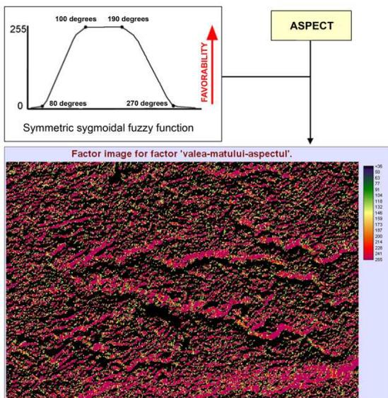
Fig. 4 - The standardization of the aspect values by using a sigmoid symmetric membership fuzzy function.
