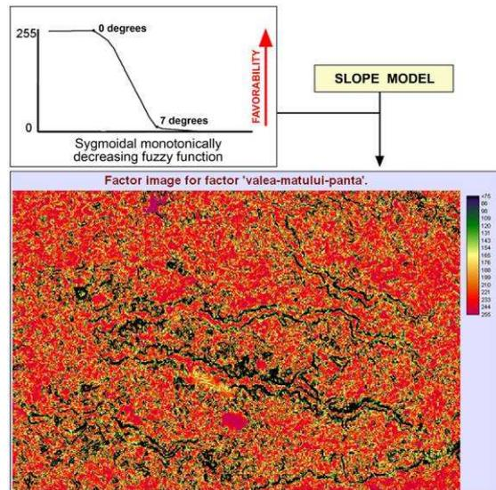
Fig. 3 - The standardization of the slope values by using a sigmoid membership fuzzy function, with monotone decreasing.
