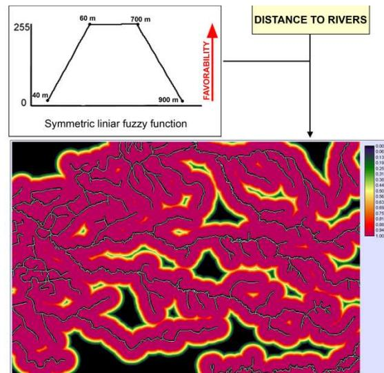
Fig. 5 - The standardization of the distances to the water by using a linear symmetric membership fuzzy function.
