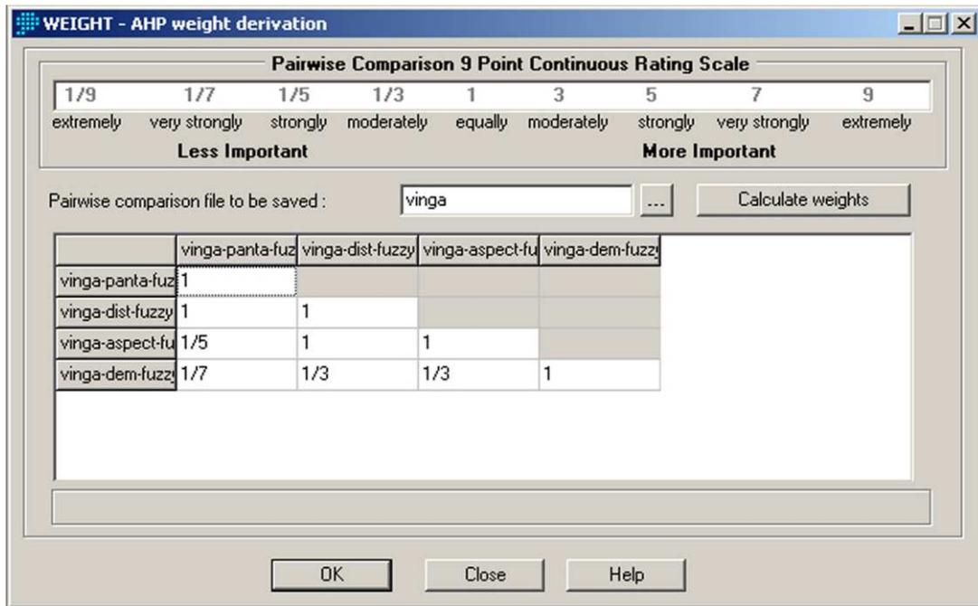
Fig. 6 - The WEIGHT module (IDRISI Andes): the nine values scale and the matrix of the scores given to the four factors, analyzed two by two.
