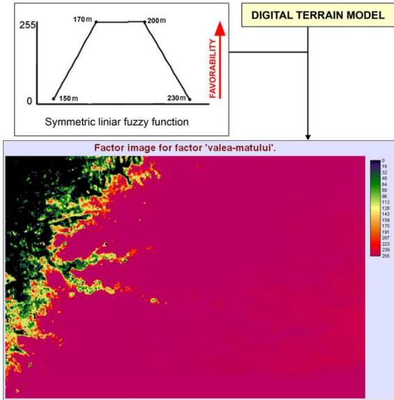
Fig. 2 - The standardization of the altitude values by using a linear symmetric membership fuzzy function.
